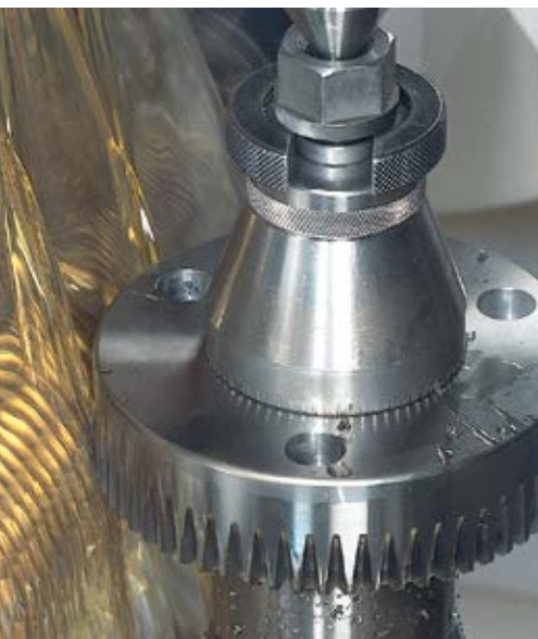
Gearing at the hobbing process
