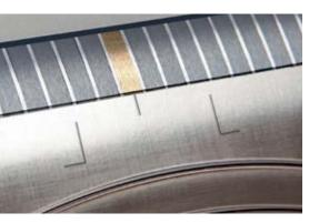
Thanks to a mark on the cylinder the exact central positioning is easily made.
