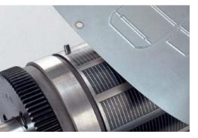
Positioning system with fit drill and dowel pin
