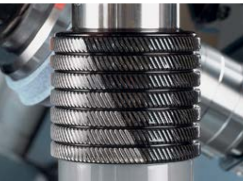
Grinding of hardened gears
