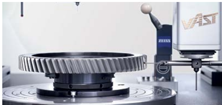
The gearing quality is checked on a 3D-measuring machine
