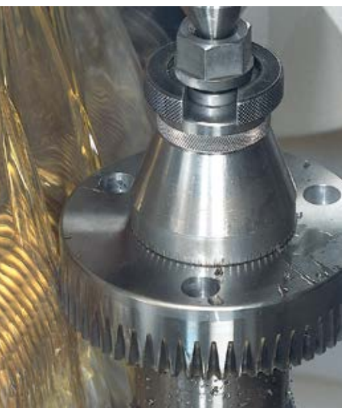
Gearing at the hobbing process
