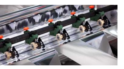
Easy installation at the grab handle. The cutting position is easily and exactly adjustable by the use of the knurled screws.
