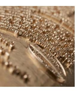
Of particular importance for the filigree stamping elements is the constant and exact tempering of the tools. According to the requirements and intended use Spilker offers oil as well as electric heated tools.
