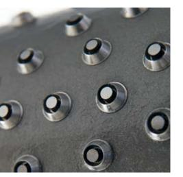
The ejector pins are mechanically ground to exactly the same height and provided with a chamfer.
