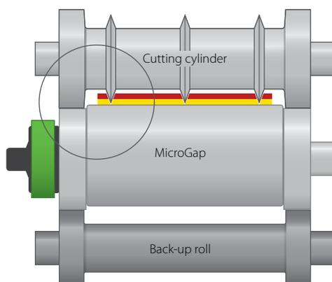
During the fine adjustment the position of the bearers does not change so that there is no need to correct the contact pressure.
