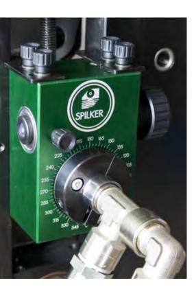
SONIC-Control allows setting up the blow-off position with an additional adjustment screw
