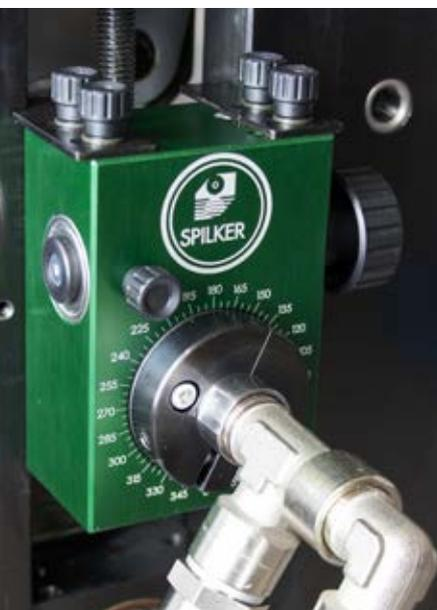
The SONIC-Control adjustment device facilitates the precise setting of the blow-off position with a knurled screw. The chosen angle can be read off on the scale and consequently be exactly reproduced for follow-up orders.
