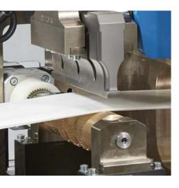
The precisely milled anvil rollers serve as counter bearings for the sonotrode and determine the welding outline.
